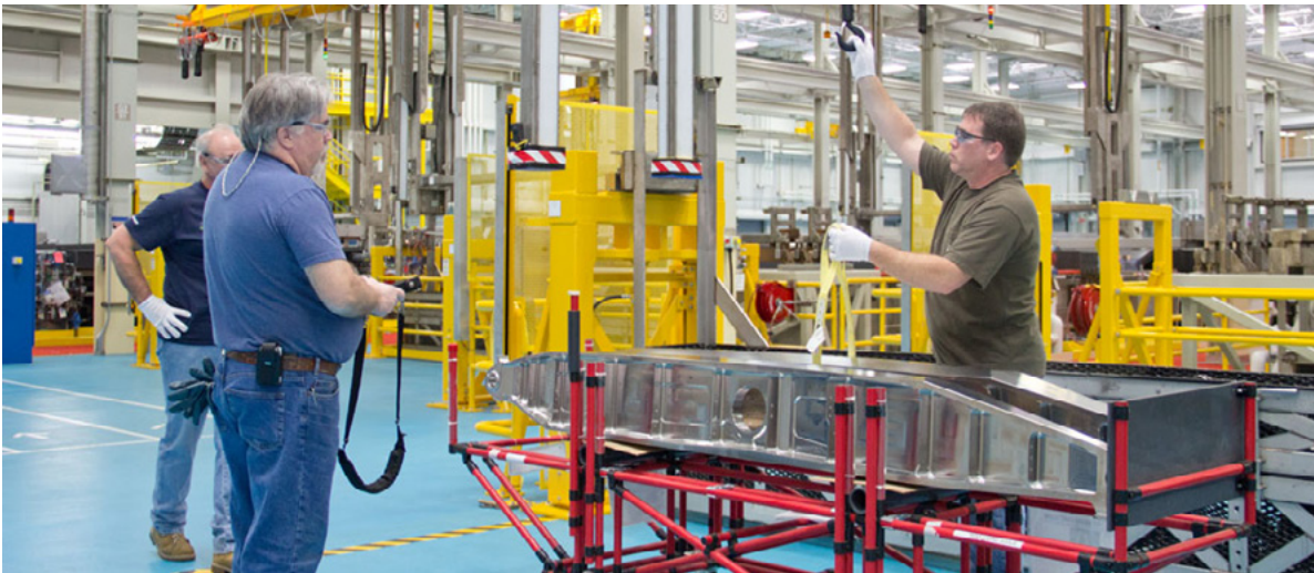
Don Williams, left, and Troy Webster prepare the first Next-Generation 737 beam for processing in the new plating facility at Boeing's Portland, Ore., site. The facility is investigating the possible use of a water-based degreasing system to reduce the use of solvents, along with other chemical-reduction strategies. (Boeing photo)
