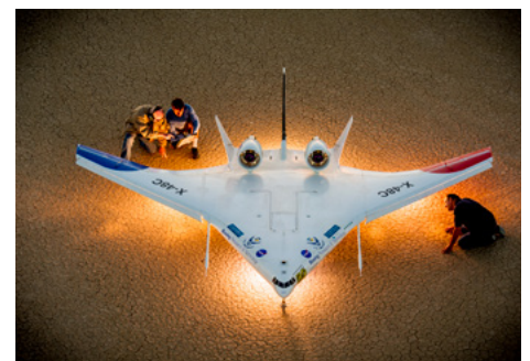
The X-48C research aircraft blends the wing and body in a new design concept that Boeing is testing to determine the aircraft's potential of significantly greater fuel efficiency and reduced noise. (Boeing photo)
