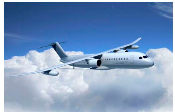
SUGAR Volt uses a hybrid electric propulsion system that can improve fuel efficiency, noise and greenhouse gas emissions. (Boeing image)
