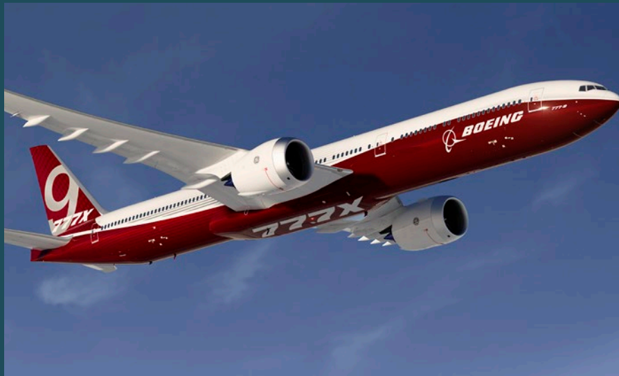
With composite wings and highly advanced engines, the 777X will reduce fuel use and emissions 12 percent over the airplanes it replaces.
