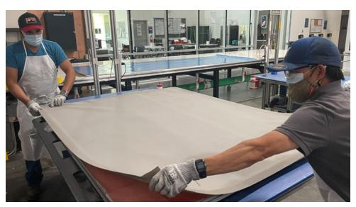
Boeing EnCore Interiors layup technicians Alberto Nieto Garcia (left) and Bang Nguyen laying out a silicone bag as part of the 737 floor panel fabrication process. The new reusable bagging system is expected to save an estimated \$175,000 annually in material costs. (David Brink photo)
