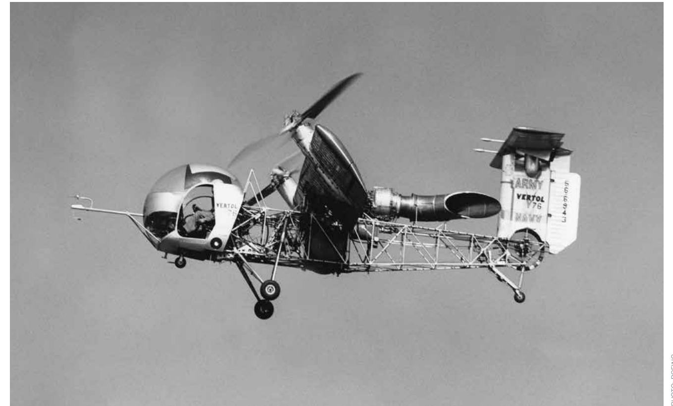
THEN: In the 1950s, the Model 76 (VZ-2) was Boeing heritage company Vertol's first move into tilt technology.
