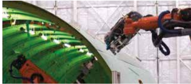
FIGURE 39. The Boeing 777 FAUB fuselage assembly process.
