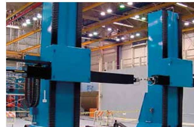
FIGURE 5A. Boeing AUSS Tower, used for NDE of large composite structure during manufacturing.
